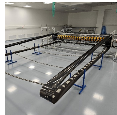
Flexible Solar Array System deployment test
