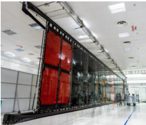
Deployed Flexible solar array sub-system
